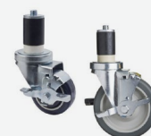
Expandable Threaded Stem Casters Grease-resistant, polyurethane non-marking wheels. Make worktables mobile. Rubber stems expand inside worktable legs for a snug fit. FECST5, FECST5B, FECST3
